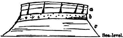
Fig. 1.—Section showing the Portland fissures. a , stone, fissured; b , sandy clay; c , shaly clay.
